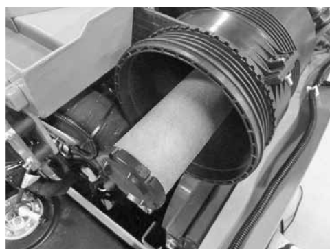
Air filter, inner screen element (replace only when necessary) 64713 (520) / 65229 (528/530)
